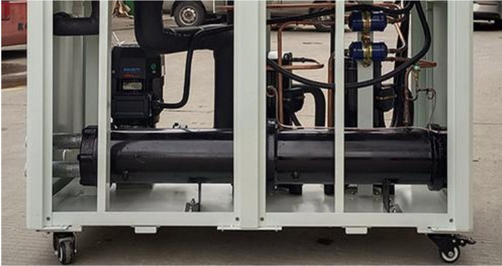
*Shell and tube Condenser for water-cooled plasma cutting chiller*
